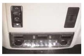
If the switch is held for more than 3 seconds, the GM interprets the continuous ground signal as a request to turn the interior light circuit off for the Workshop Mode as on previous systems. The workshop mode is stored in memory and will not come back on even if the GM is removed from it's power supply and reconnected. The switch must be pressed to turn the lights back on.
